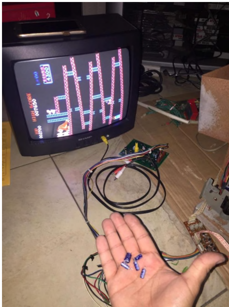
Picture 2. Producing a clean, color-stable signal from the two-bit convertor after replacing parts (Old capacitors held in hand).
