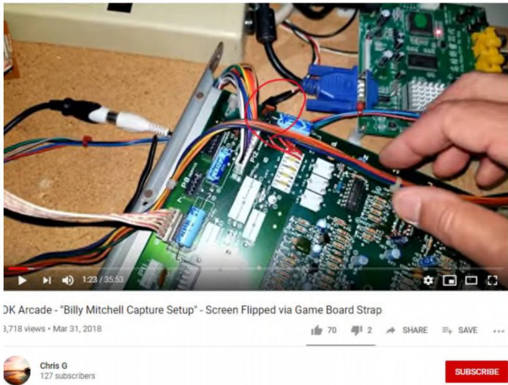
Picture 4. A picture of the orientation switch proposed by David Race and tested by Chris Gleed. The switch is the orange and black piece circled in red.
