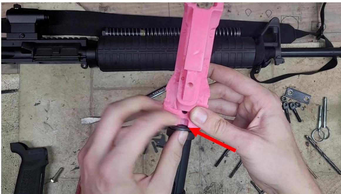
*Ensure that the nub on the locking plate aligns with this cutout in the lower. Tighten the castle nut enough to keep it from coming loose, but do NOT tighten it down to mil-spec.*
