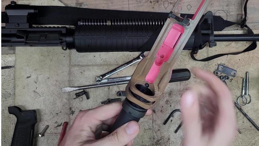
*Screw the tube in just enough to keep the retainer from falling out, while ensuring the tube is more or less straight (the lug on the bottom of the tube which the stock locks onto should be at the bottom of the tube).*
