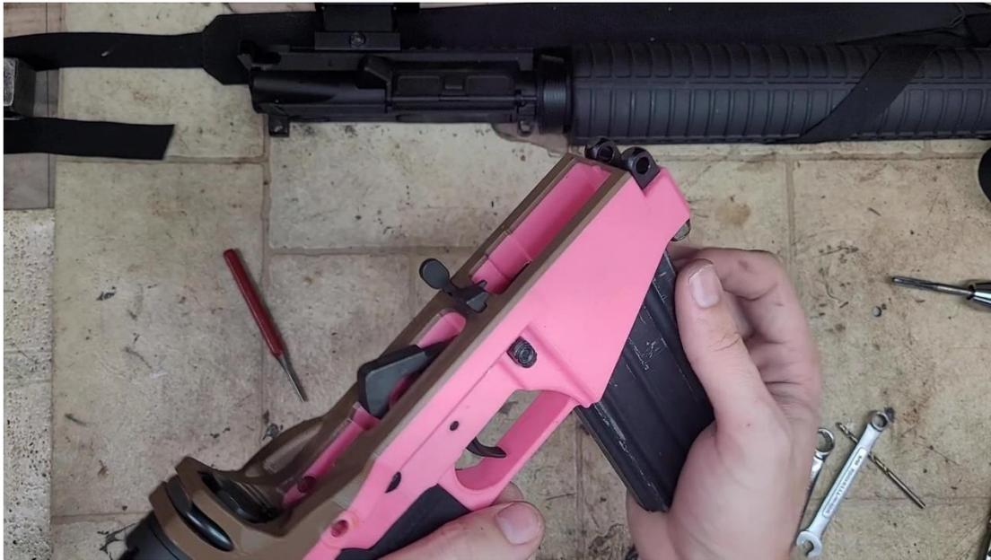
*You can check magazine fitment now – they should slot in easily and drop free, assuming your print settings were good and you removed all your supports. If your printer exhibits ringing or z-banding, you may need to do some light sanding on the front and rear faces of the magwell – it is designed to be a perfect fit with a perfect print, and has no added tolerance for rough prints.*
