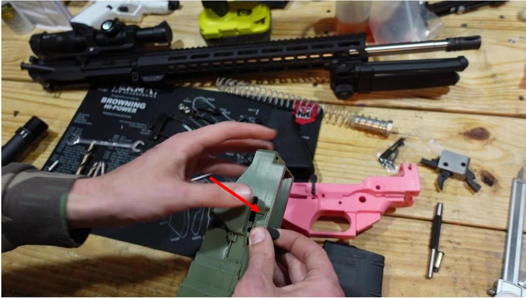
*Place the roll pin into its trough*
