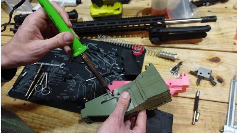
*How to remove a stuck/sticky bolt catch plunger*
