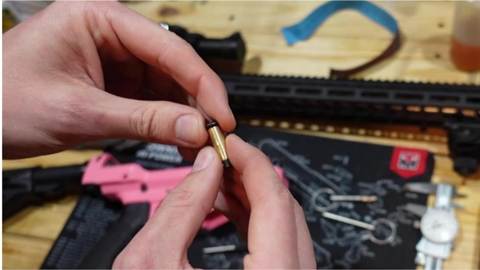
*Using an AR15 takedown pin as an installation tool for the bushings is recommended!*
