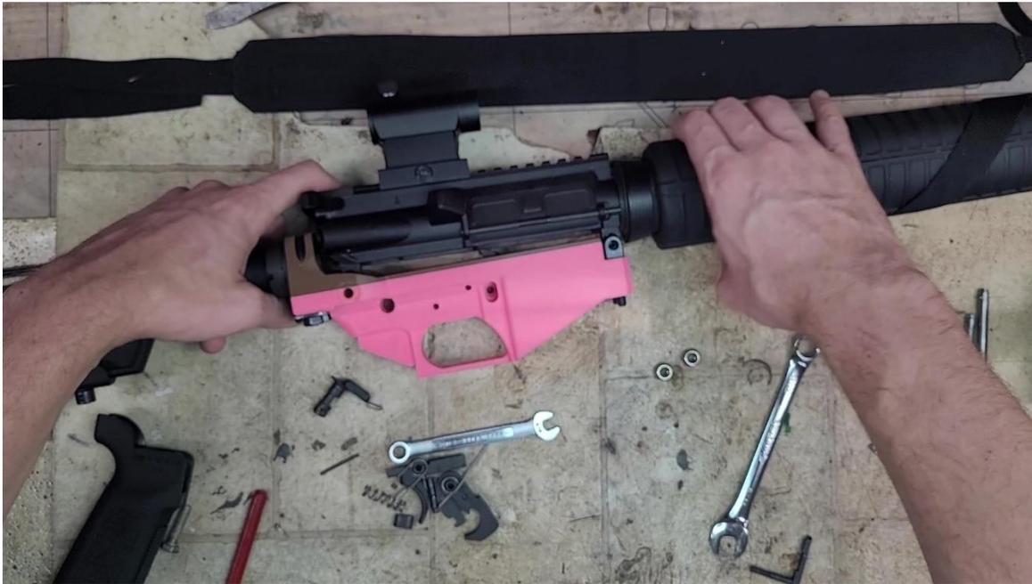
*Mate your upper and lower receivers. Make sure that the eye bolts are not tightened down yet! They should be able to rotate to allow the upper to fit.*
