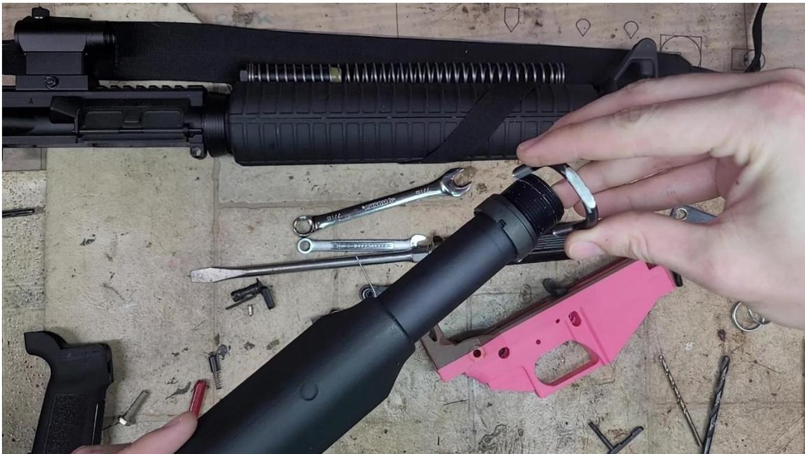
*Test the fit between the u-bolt and buffer tube. Out of the box, the u-bolt will not be able to sit down on top of the tube – you will need to clearance the u-bolt so that it can sit down on the tube.*
