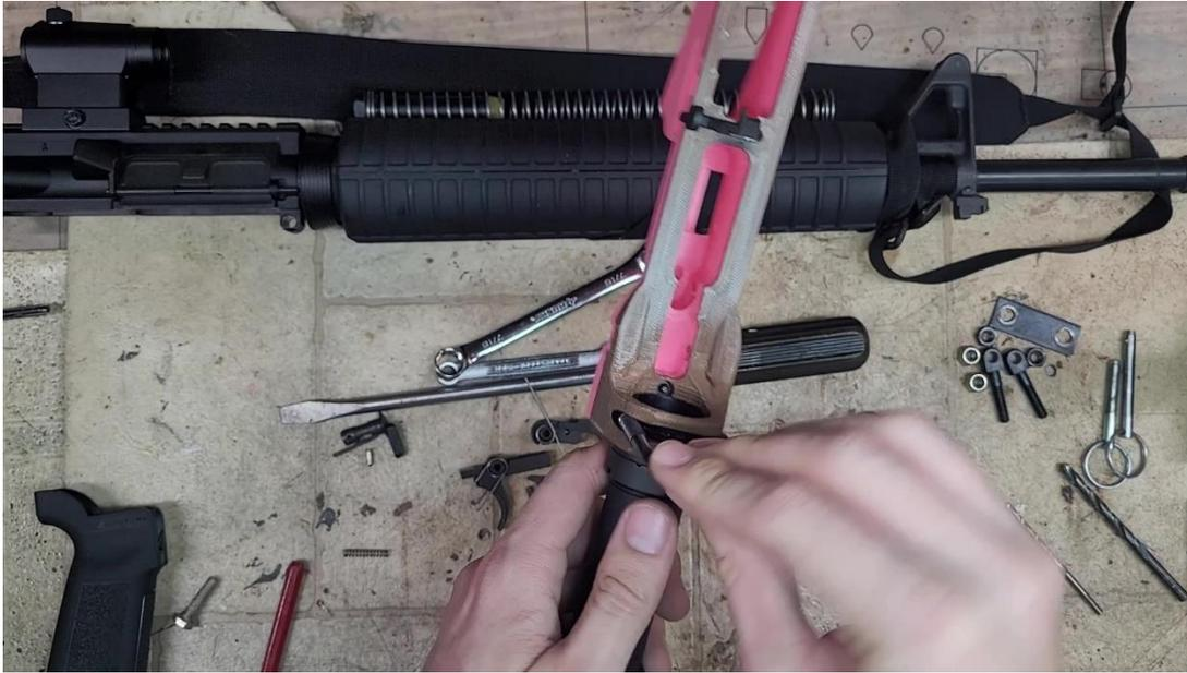
*Install the u-bolt. You may have to gently tap the bolt to get it into place, but it shouldn't take much force. If it feels like it needs to be hammered into place, ensure that your u-bolt legs are not bent out of shape and clearance the parts further.*
