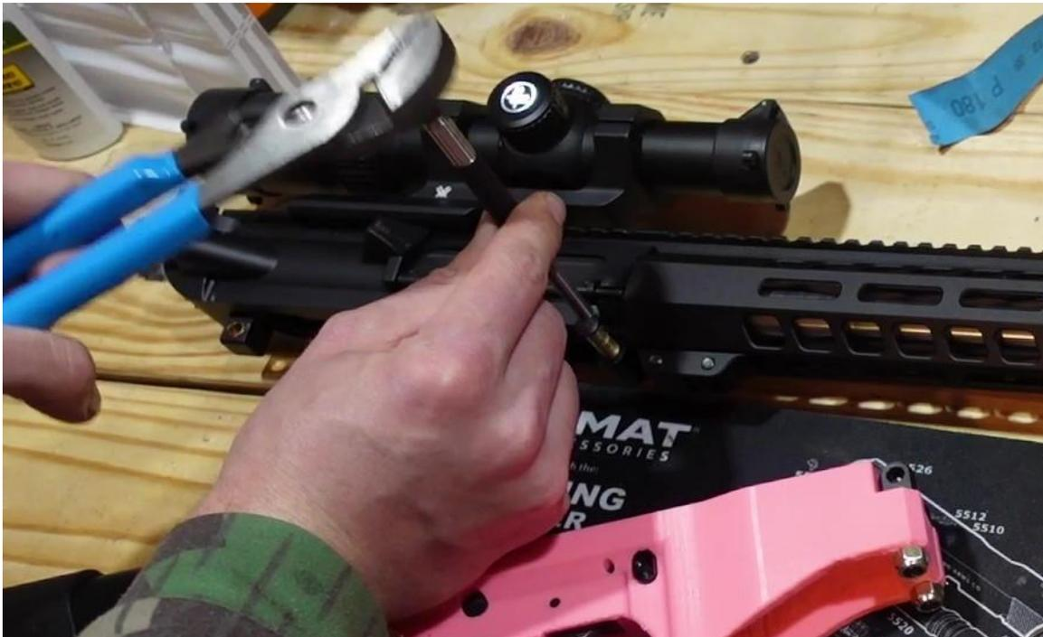
*Using the AR15 takedown pin as a tool, you can tap on the head of the pin to seat the bushing into the upper. Perform these steps for both bushings, and once the bushings are inside the lugs on the upper, you are ready to proceed.*
