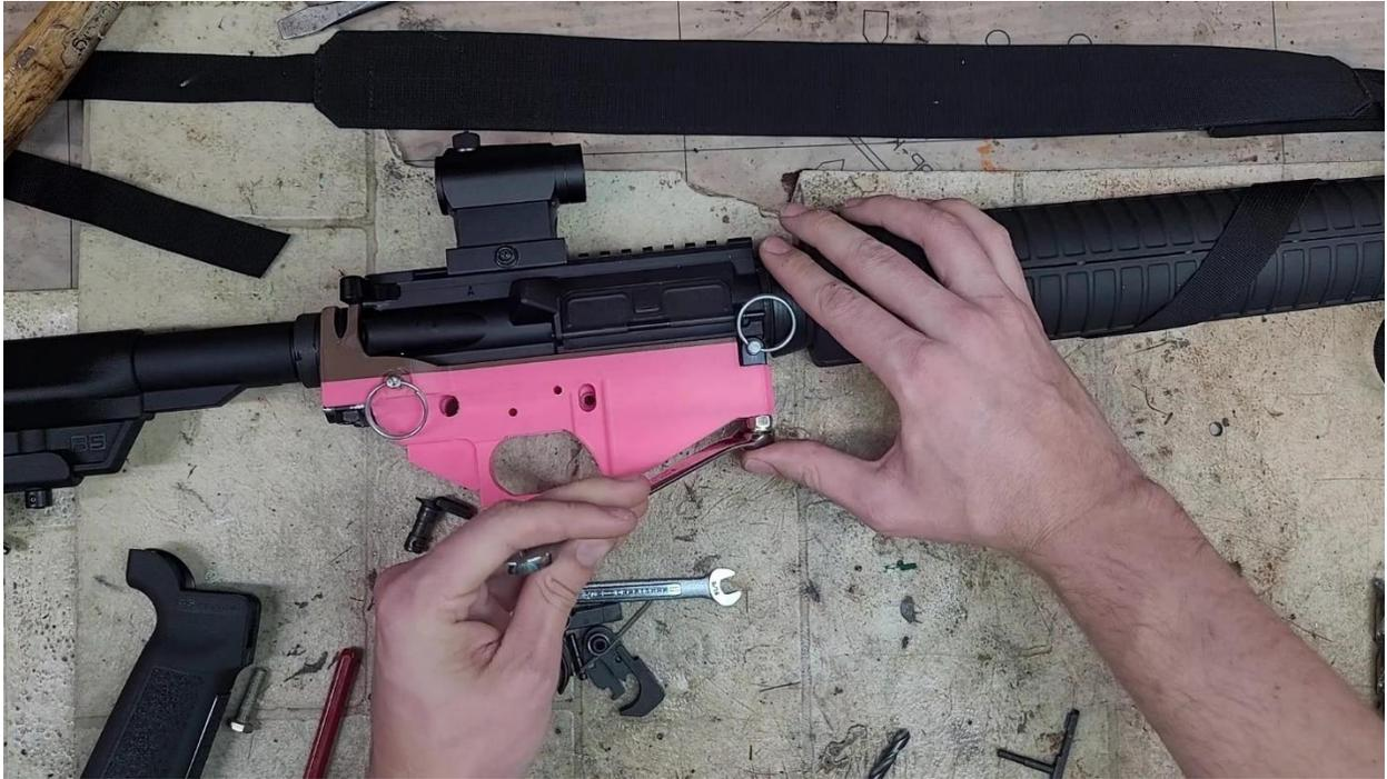
*Use your 7/16" wrench to tighten the nuts on the eye bolts. Don't make things so tight that the pin becomes very hard to remove, but don't leave any gap between the nut and the bottom of the lower.*
