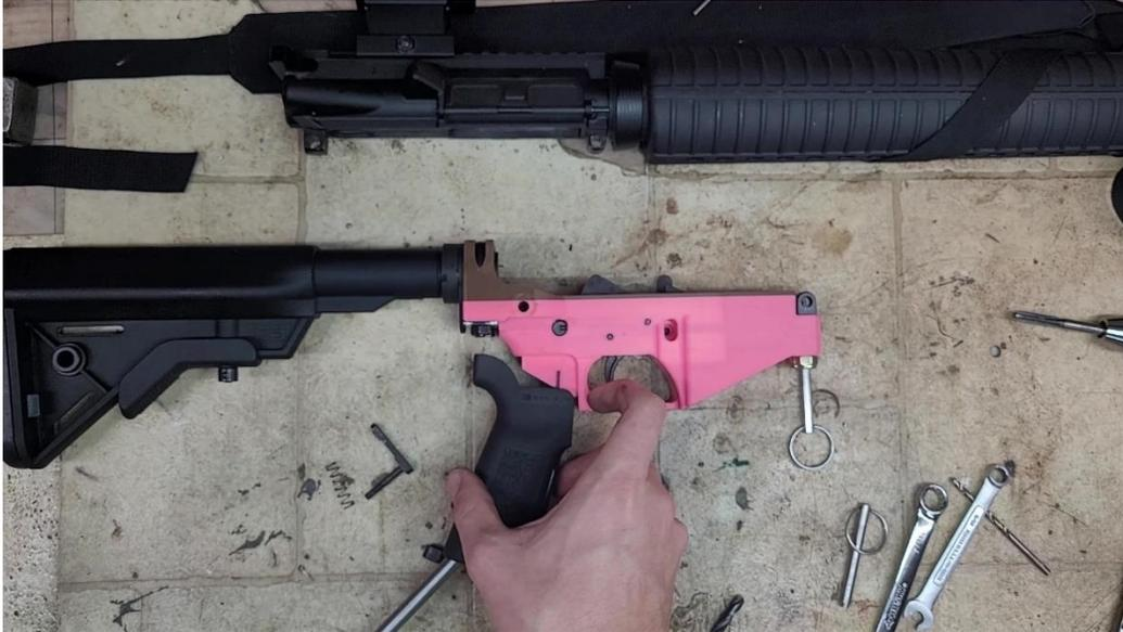
*Install the safety, detent, spring, and pistol grip. Standard AR lower building operation.*
