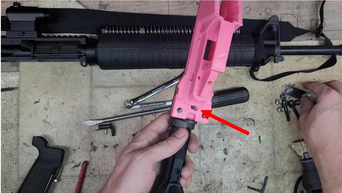
*Install the buffer retainer spring into this hole – the underside of the hole you already put the buffer retainer into.*
