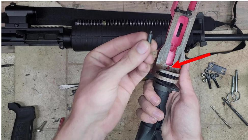
*Place the retainer into this hole before you screw the tube in fully. Do not install the retainer spring yet.*
