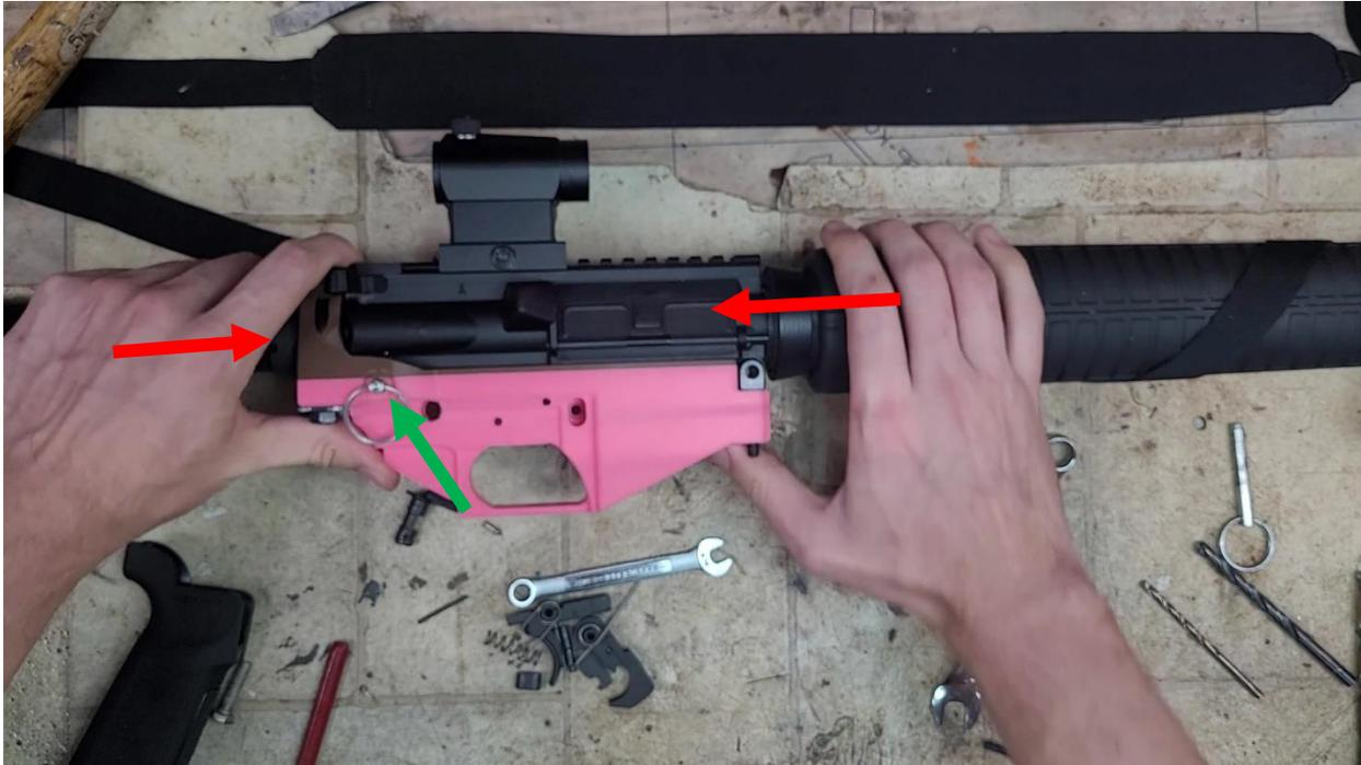
*Make sure that the upper and lower receivers are pushed together, then stick your rear takedown pin into place. It might be tight when you first insert it – it will loosen up some over time, but if you can't stand pins being tight then you can oil the pin, or sand the pin down a little.*
