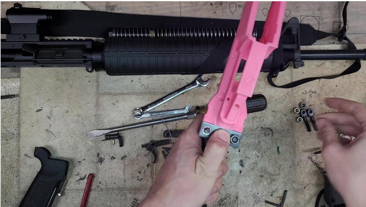
*Install nut plate and nuts. Use a 7/16" wrench to tighten these nuts.*
