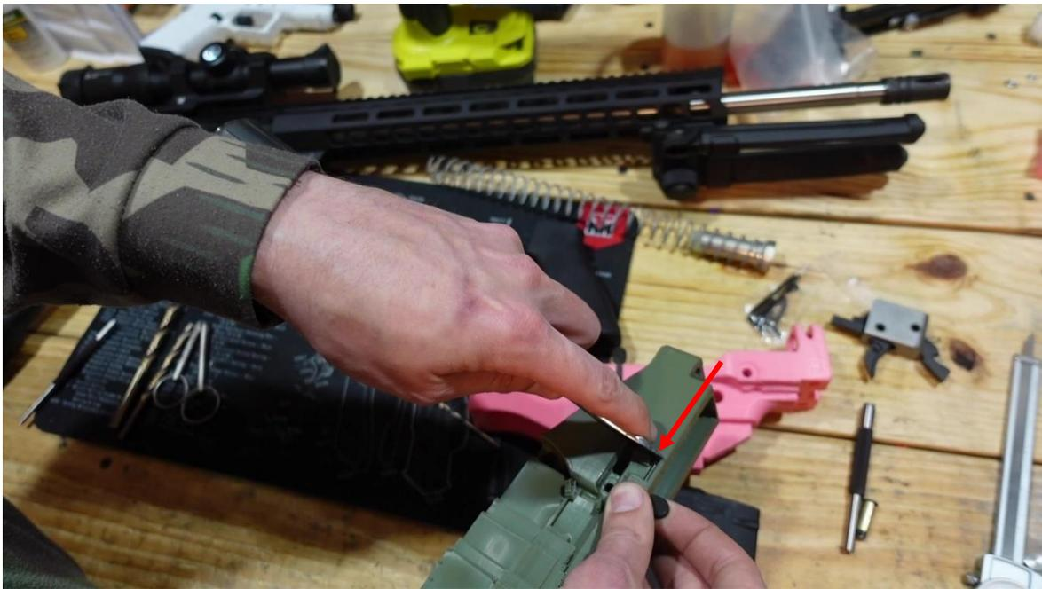
*Use a screwdriver to push the roll pin into place while holding the bolt catch in alignment with the hole.*
