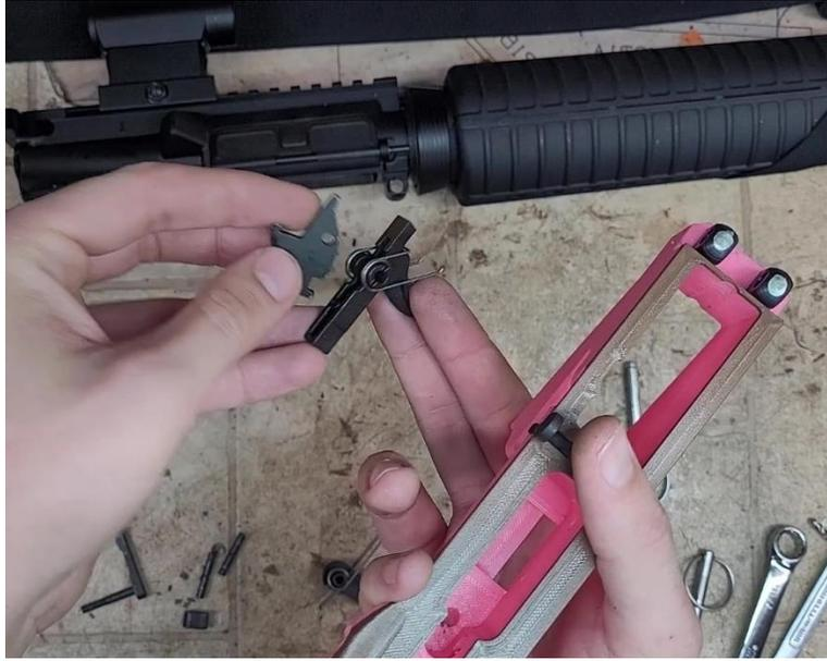
*Install the trigger and disconnect*
