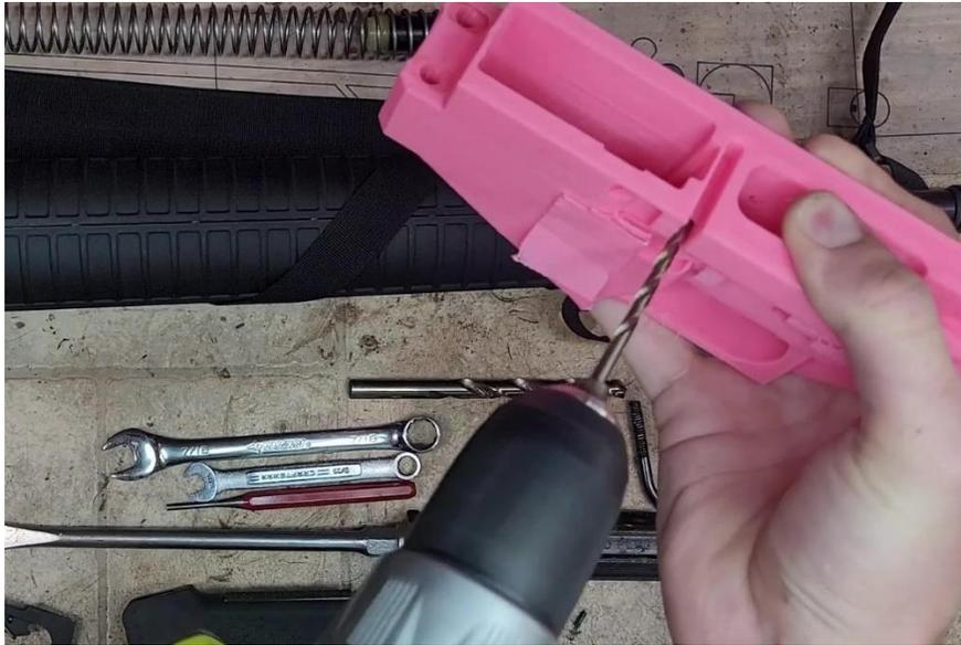
*Clean out the bolt catch spring plunger hole with a 5/32" drill bit.*
